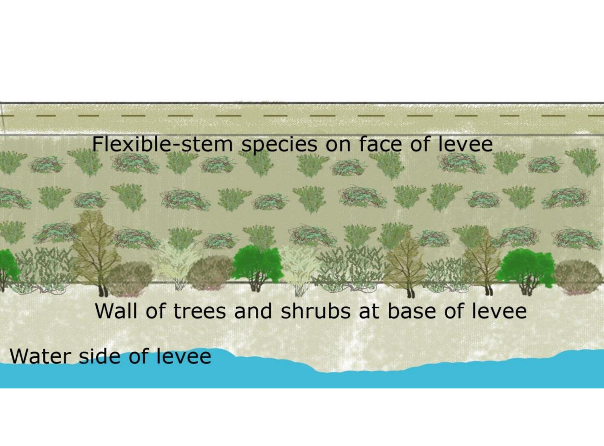
A cross-sectional diagram of a levee. At the top is a road with a dashed center line. Below the road is a thick layer of soil. The middle section shows a dense layer of small, green, flexible-stemmed plants. At the base of the levee is a layer of larger trees and shrubs. The bottom of the diagram shows a blue area representing water.
