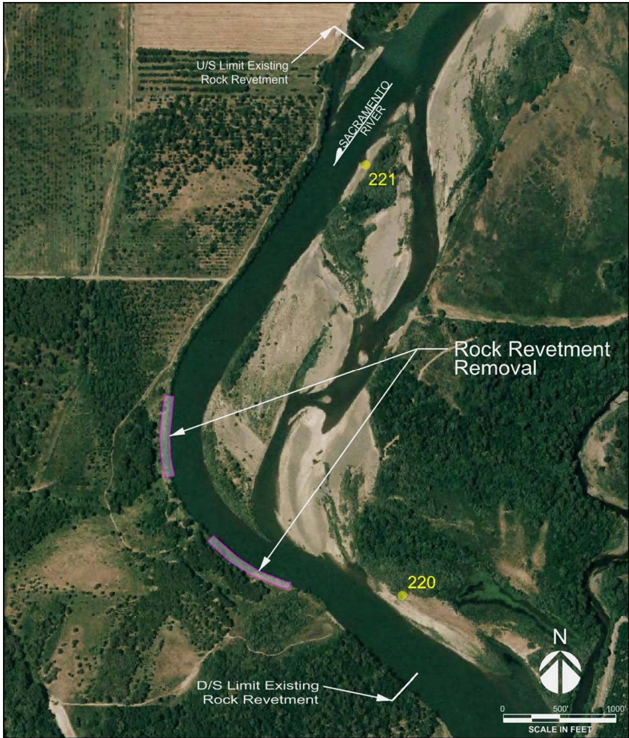
Figure 7. Half Length Notching Rock Revetment Removal
