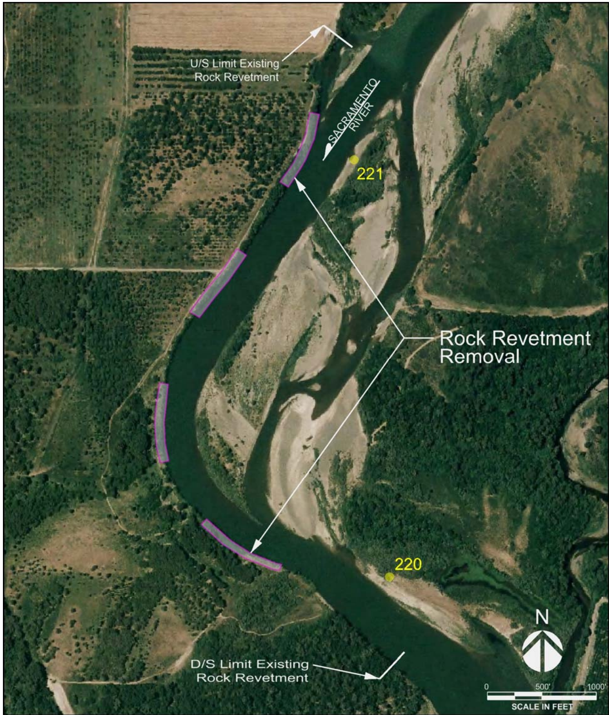
Figure 6. Full Length Notching Rock Revetment Removal
