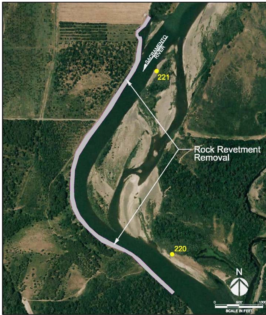
Figure 28. Location of Rock Revetment Removal
