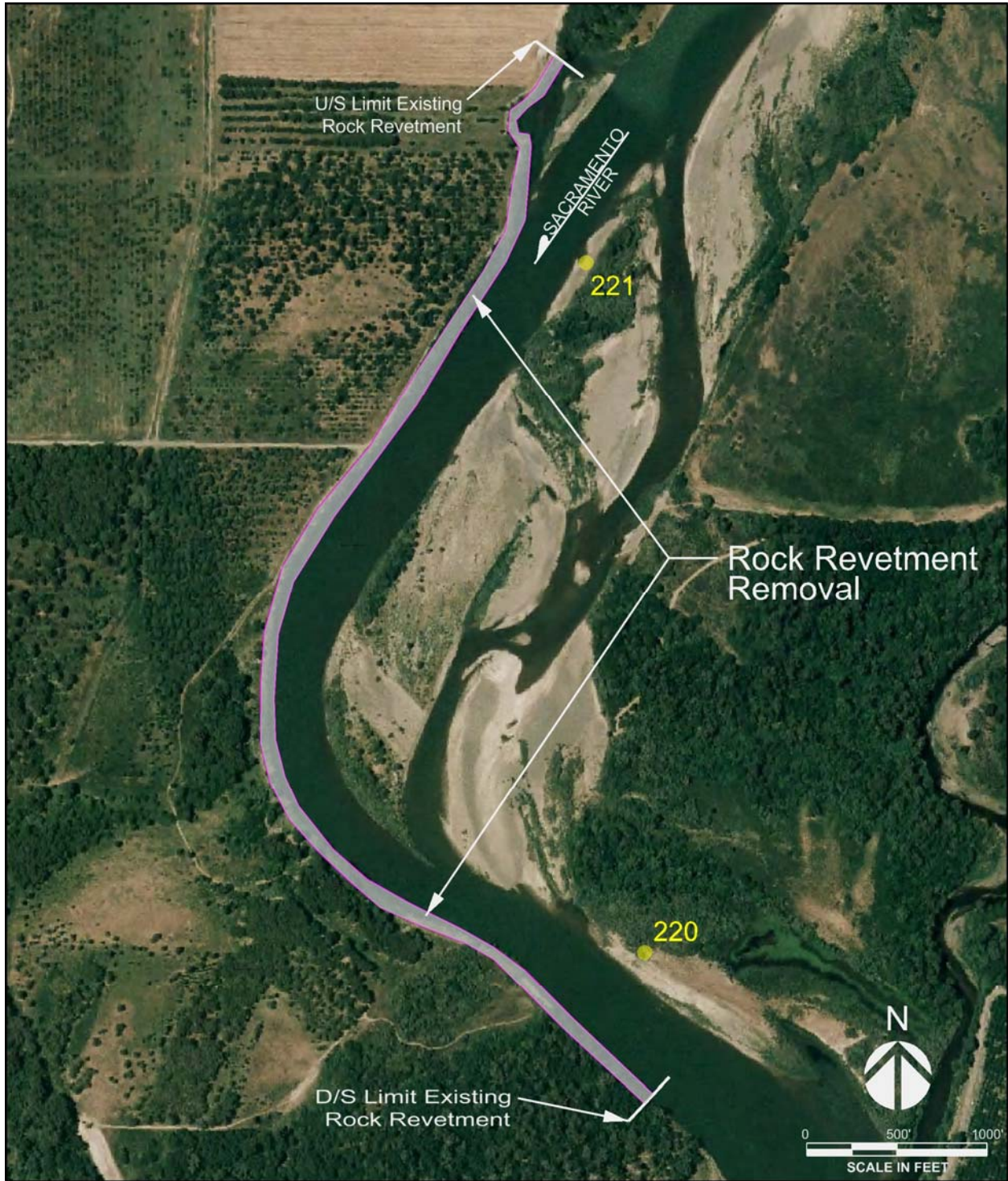
Figure 4. Full Length Rock Revetment Removal
