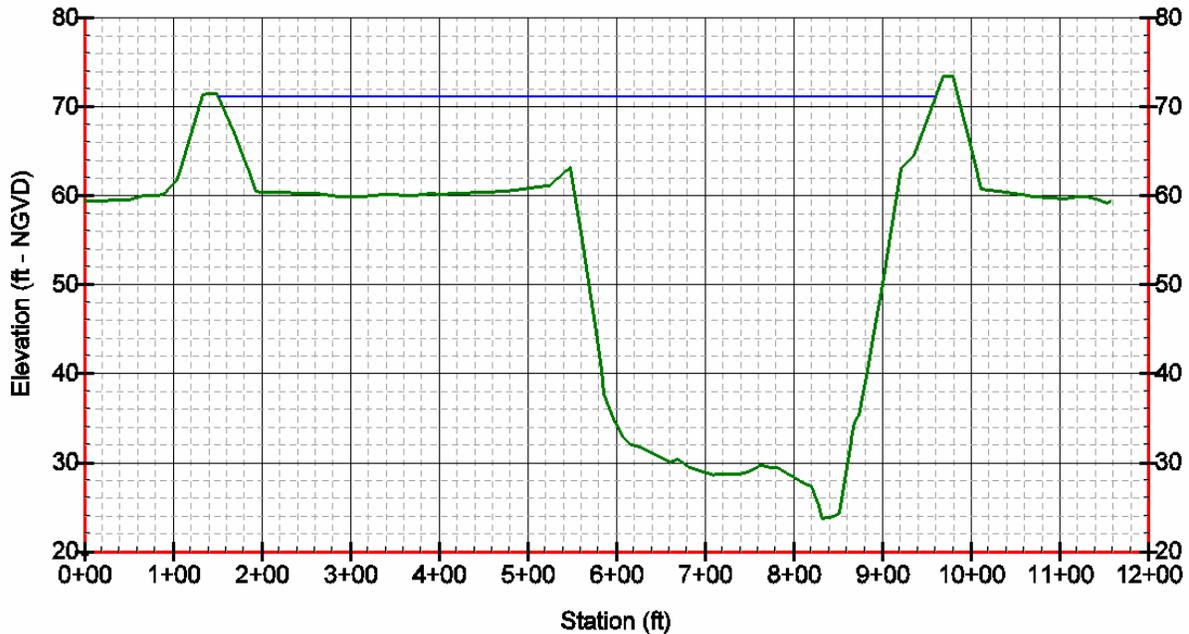
**Figure 10. Cross Section of the Sacramento River, just Upstream of Colusa Bridge with Water Surface Elevation Corresponding to a Flow of 65,000 cfs**
