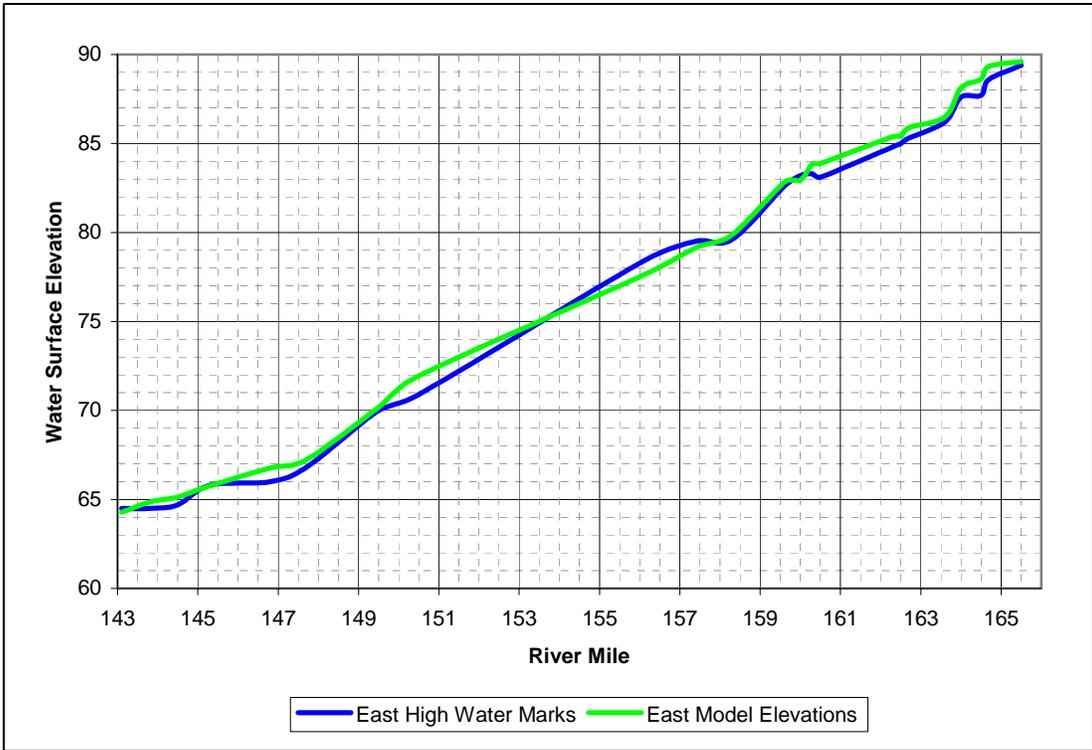
**Figure 11. Profile Comparison of High Water Marks on the East Bank**
