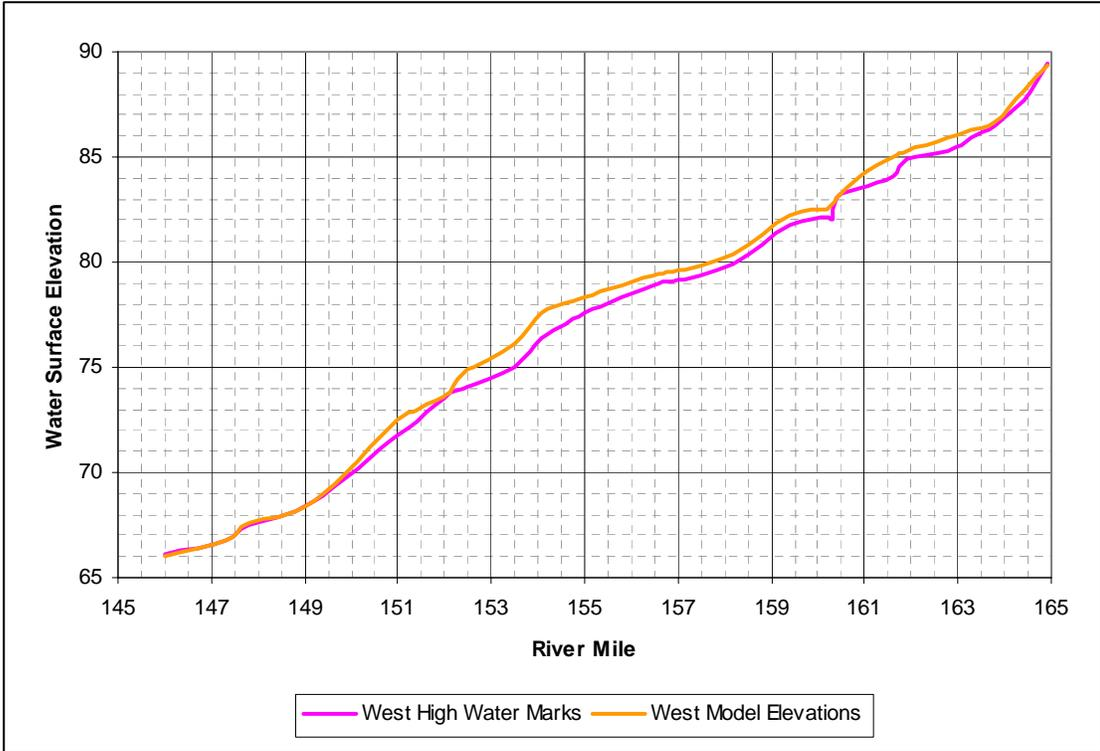
**Figure 12. Profile Comparison of High Water Marks on the West Bank**
