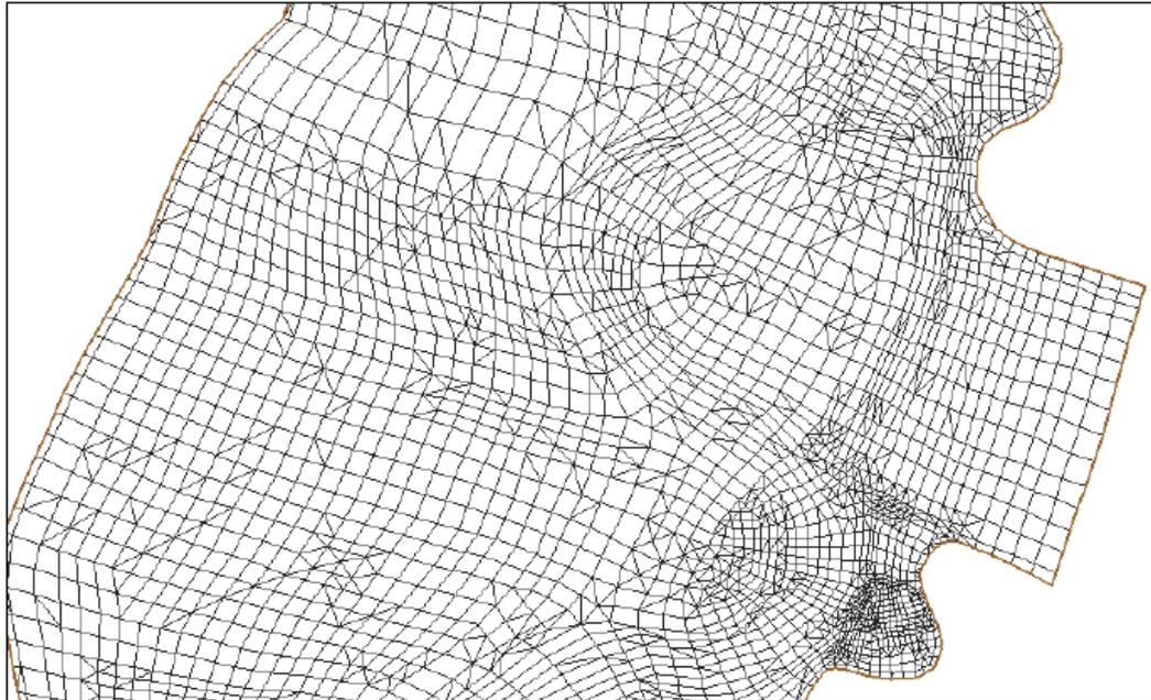
**Figure 6: Example of finite element mesh (Ayres Associates)**
