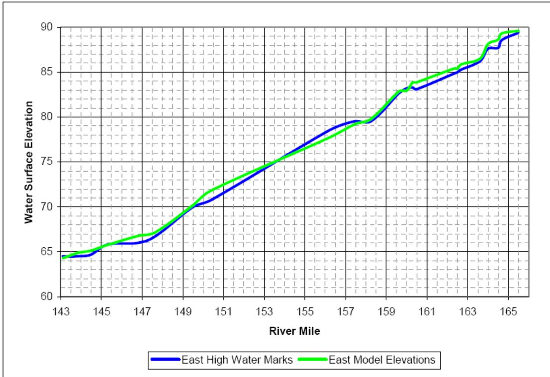
**Figure 3: Comparison of Modeled Water Surface Profile with High Water Marks on the East Bank. (Ayres Associates) Note that model calibration trends at or slightly above the measured high water marks at most locations, including the vicinity of Ward Tract (RM 145 to RM 146)**
