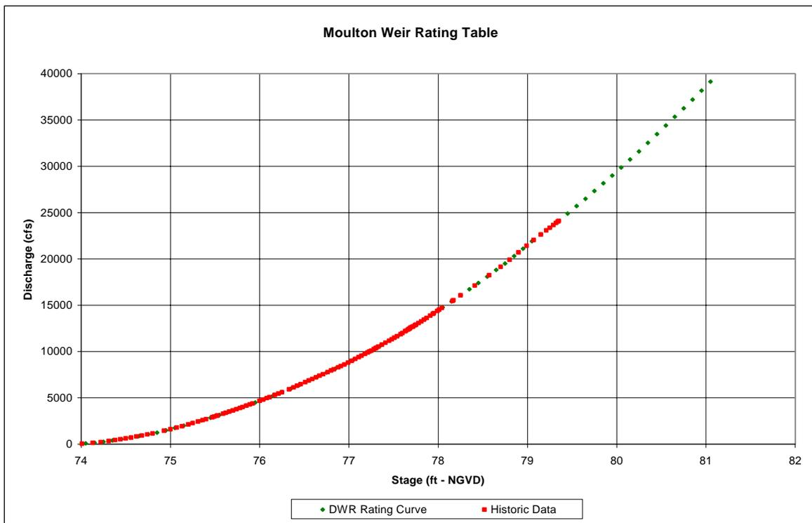
**Figure 8. Rating Curve at Moulton Weir**
