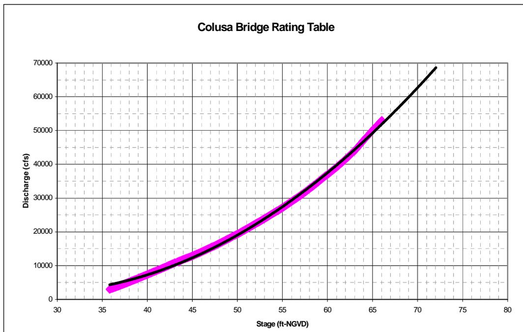
**Figure 9. DWR Rating Curve at Colusa Bridge**
