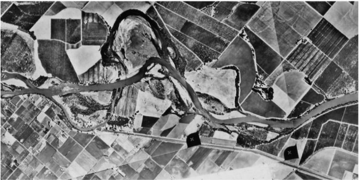
Figure 2. During the 1970 flood, an eastward meander bend cut off by chute cutoff, resulting in channel downcutting of appx 3 ft at the bifurcation point between the main channel and a side channel maintained to serve as the point of diversion for the Glenn-Colusa Irrigation District Canal.
